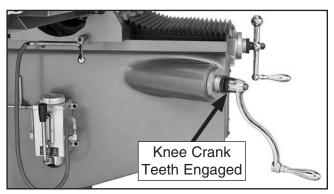
Figure 11. Knee crank teeth engaged.
